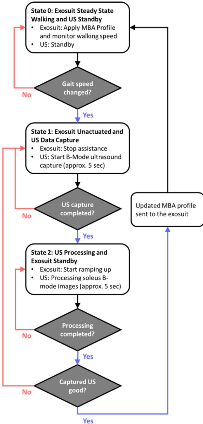
**Fig. S5. Finite State Machine diagram for real-time on-demand MBA profile generation.**
