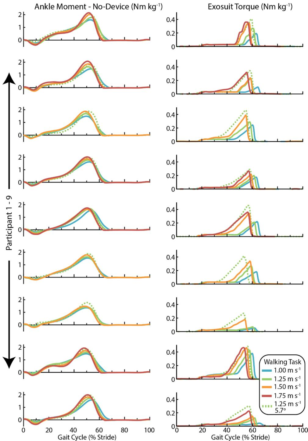
**Fig. S2. Ankle moment and applied exosuit torque with the MBA profile for each participant.** Two individuals did not complete  $1.75 \text{ m s}^{-1}$  and the GRF data were unusable (belt crossover) for one individual at  $1.75 \text{ m s}^{-1}$ .
