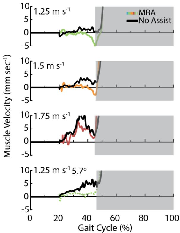
1000 **Fig. S4. Measured muscle velocity with and without MBA assistance.** The gray region represents an area of measurement uncertainty where the ankle begins plantar flexion and high actuator force may cause movement in the probe.
