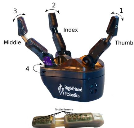
Fig. 1. Top: The underactuated hand used here has four actuated degrees of freedom – three for finger flexion, one for coupled rotation of two fingers to transition between wrap grasps and pinch grasps. Bottom: Barometer-based tactile sensors molded into finger contact surface.
