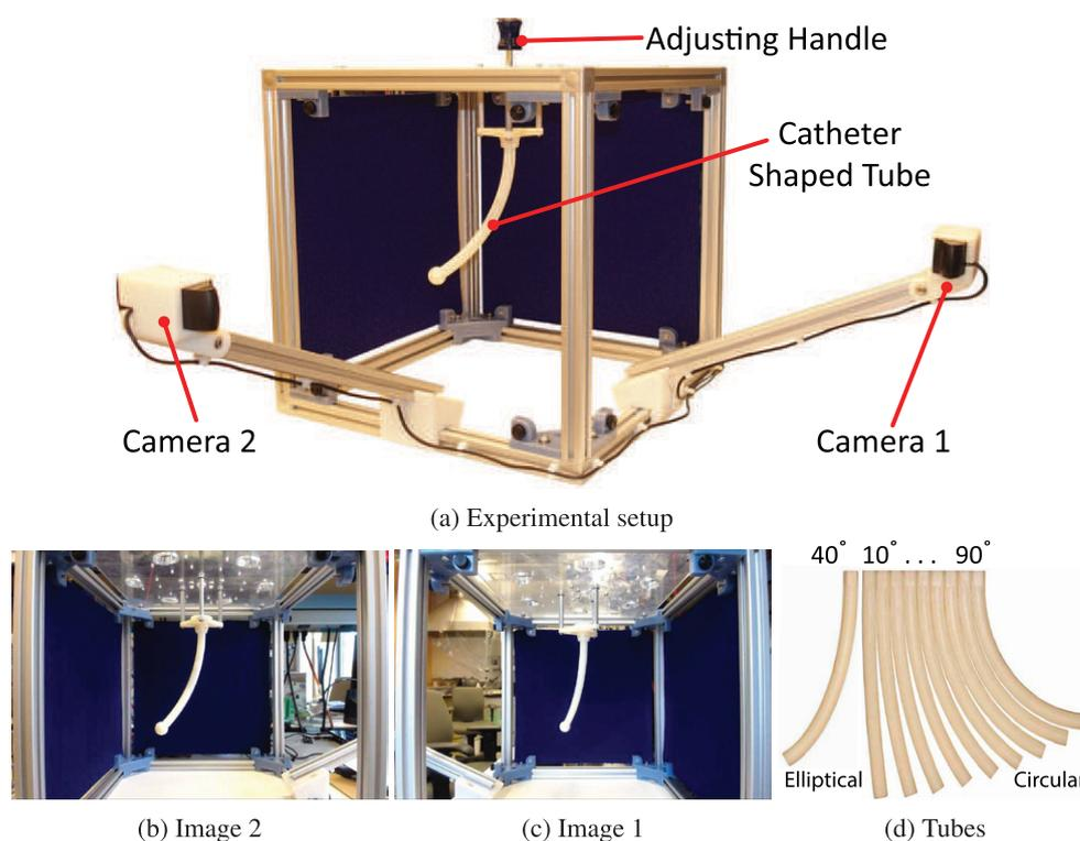
**Figure 3.** Developed system for evaluation of the proposed 3D reconstruction algorithm, examples of the images from both cameras and 3D printed circular and elliptical catheter shaped tubes with known shape. (a) Experimental setup. (b) Image sample from camera 2. (c) Image sample from camera 1. (d) Tubes.
