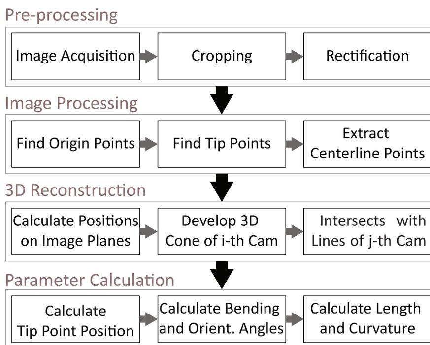
Figure 2. Block diagram of the proposed high speed vision-based algorithm for catheter 3D reconstruction.
