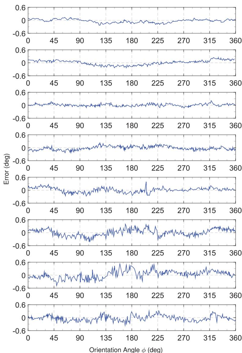
**Figure 9.** Measurement errors of the bending angles in the second experiment for the circular tubes with the bending angles of 10–70 deg and the elliptical tube respectively from top to bottom.
