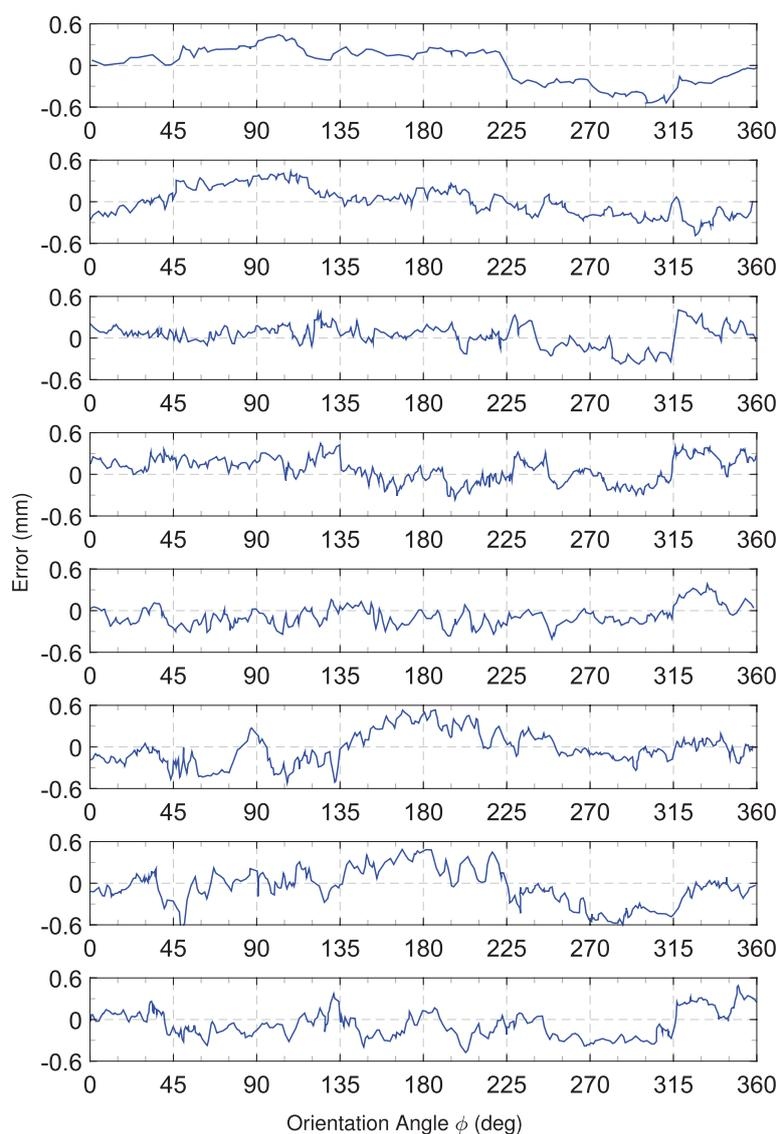
**Figure 8.** Measurement errors of  $z$  coordinate of the tip point in the second experiment for the circular tubes with the bending angles of 10–70 deg and the elliptical tube respectively from top to bottom.
