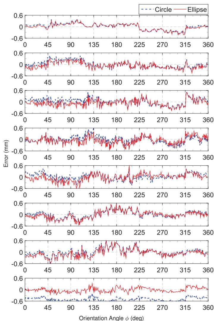
**Figure 10.** Errors of the tube lengths calculated in the second experiment based on the circles and ellipses fitted to the centerline points for the circular tubes with the bending angles of 10–70 deg and the elliptical tube respectively from top to bottom.
