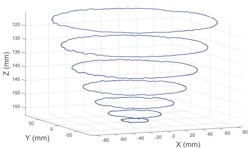
**Figure 11.** Tip point trajectories measured in the second experiment for the 10–70 deg circular tubes.
