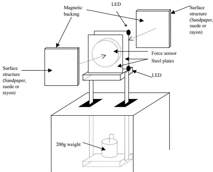
Figure 2. Experimental setup for precision grip
