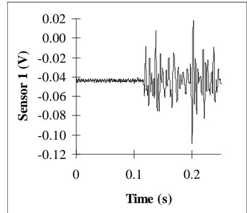
**Figure 5.** Sensor 1 output during the initiation of a wrist movement. The sensor is sensitive to wrist movements, however, the signal-to-noise ratio remains high and adequate for the tasks performed.
