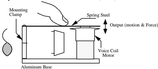
**Figure 3.** The vibrotactile display. The display mounted on the existing master controller did not require any modifications of the master controller.
