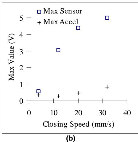
**Figure 6.** Varying gripper closing speeds. The mean frequency of the signal spectrum (a) and its maximum (b) of both the sensor and accelerometer signals increased with increasing sensor speed.
