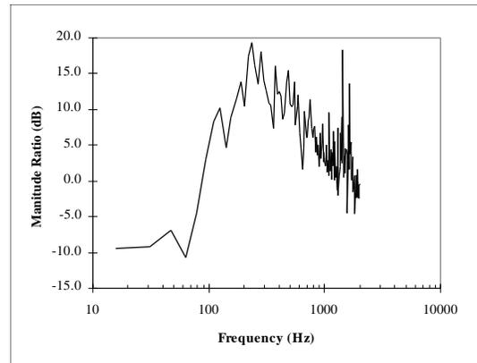
**Figure 7:** The estimated transfer function of the vibrotactile system. The transfer function input was the sensor signal and the output was the signal of the accelerometer mounted on the display
