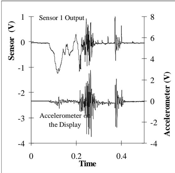
**Figure 4.** Sensor and display accelerometer output during a grasping task. The sensor contains lower frequency components than the display, but follows the sensor well at higher frequencies
