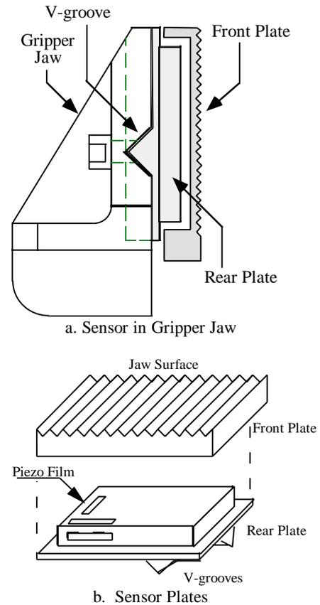
**Figure 2.** Sensor design. The rear plate of the sensor bolts onto the jaw of the remote manipulator. Between the two plates is a compliant rubber which contains the piezoelectric film.
