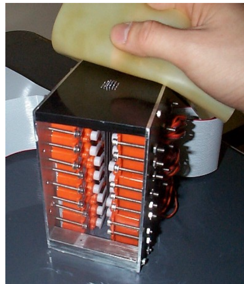
Figure 1. Pin actuated tactile display
