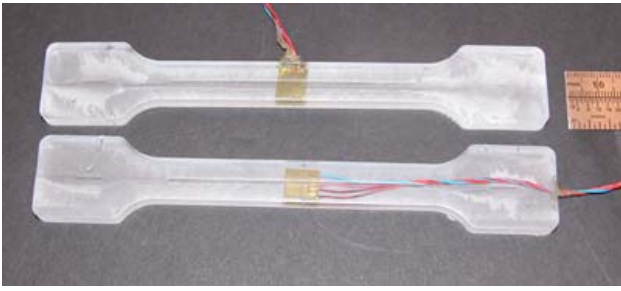
Fig. 6 Metal film strain gages embedded in beam with side-exit wires (top) and axial-exit wires.
