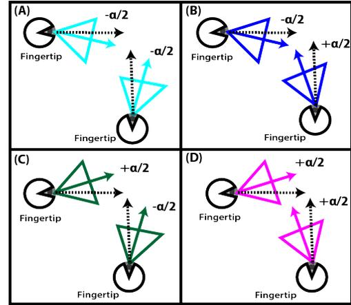
Fig. 6: There are two possible extreme contact normal vectors for a single planar contact:  $+\alpha/2$  and  $-\alpha/2$  surrounding the true contact normal. This results in four combinations of the extreme friction cones for a 2-finger planar grasp.
