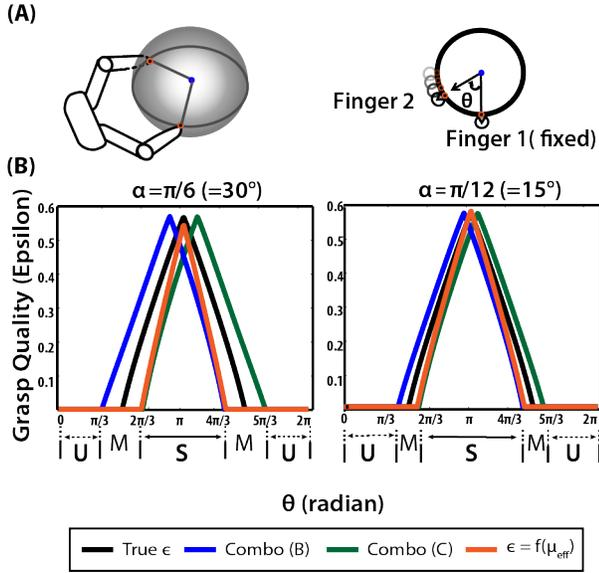
Fig. 7: (A) The  $\epsilon$  values for all contact locations calculated by fixing one finger at the bottom of the circle, and scanning the second finger along the perimeter. (B) the variability of  $\epsilon$  increases with lower sensor spatial resolution. The regions of definite stable(S), definite unstable(U), and ambiguous(M) contact locations are labeled along the bottom. Values where  $\epsilon < 0$  are unstable and are plotted as  $\epsilon = 0$ .
