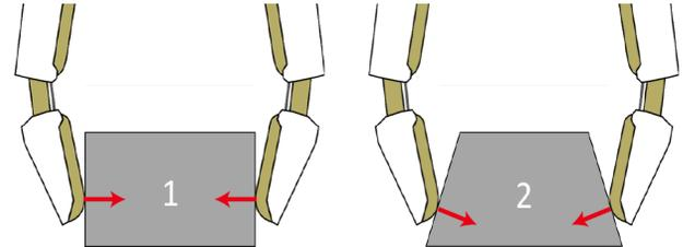
Fig. 1: Robot hand using two-fingered pinch grasp. With a moderate coefficient of friction objects 1 and 2 can both be stably grasped. If, however, the contact sensors in the robot fingertip lack sufficient resolution, then the surface normal direction for object 2 may be so uncertain that grasp stability cannot be reliably predicted.
