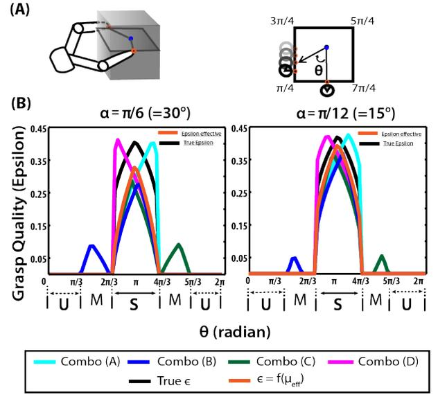
Fig. 9: (A) The  $\epsilon$  values for all contact locations calculated by fixing one finger at the bottom of the square, and scanning the second finger along the perimeter. (B)  $\epsilon$  calculated by using the four combinations of extreme friction cones shown in fig. 6. The regions of definite stable(S), definite unstable(U), and ambiguous(M) contact locations are labeled along the bottom. Values where  $\epsilon < 0$  are unstable and are plotted as  $\epsilon = 0$ .
