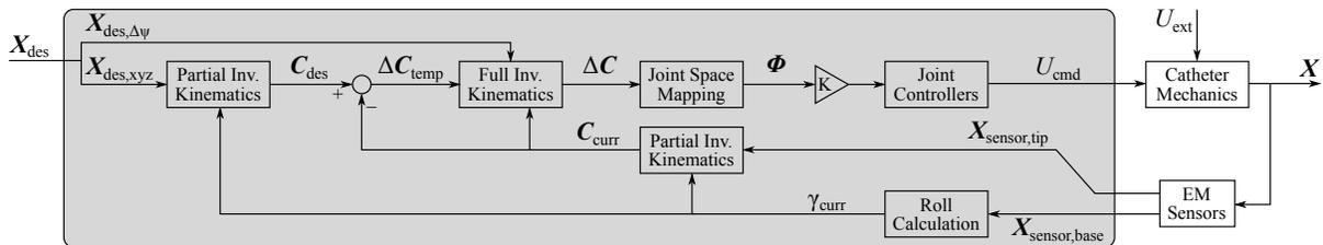
Fig. 8. The controller (gray box) receives the desired catheter tip pose and iteratively calculates joint angle adjustments to manipulate the catheter.
