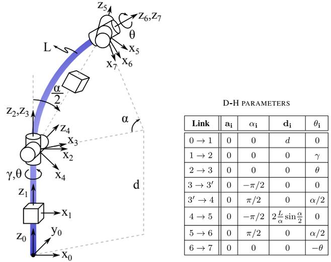
Fig. 5. Symbolic representation showing D-H parameters: translation,  $d$ , catheter handle roll,  $\gamma$ , bending plane angle,  $\theta$ , bending angle around the global  $z$ -axis,  $\alpha$ , length of the bending section,  $L$ .
