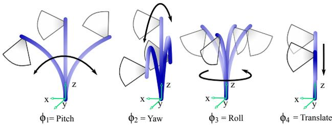
Fig. 2. Joint inputs and corresponding tip motions.
