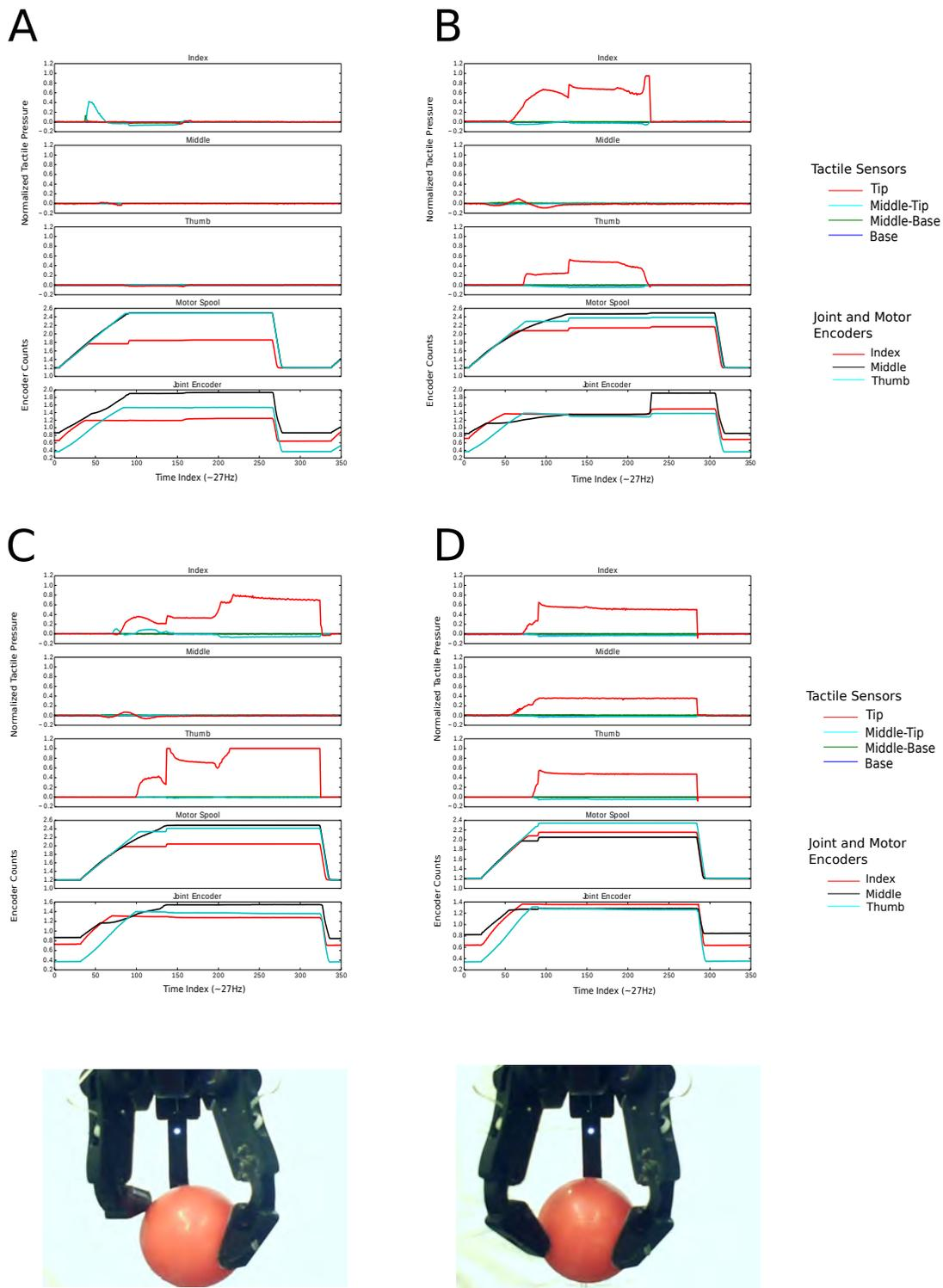
Figure 3: Sensor signals for typical examples of four cases. A: Clear failure case; B: Marginal failure case; C: Marginal success case; D: Clear success case. End-of-trial evaluation photographs are shown for successful cases C and D to illustrate hand-object configuration.
