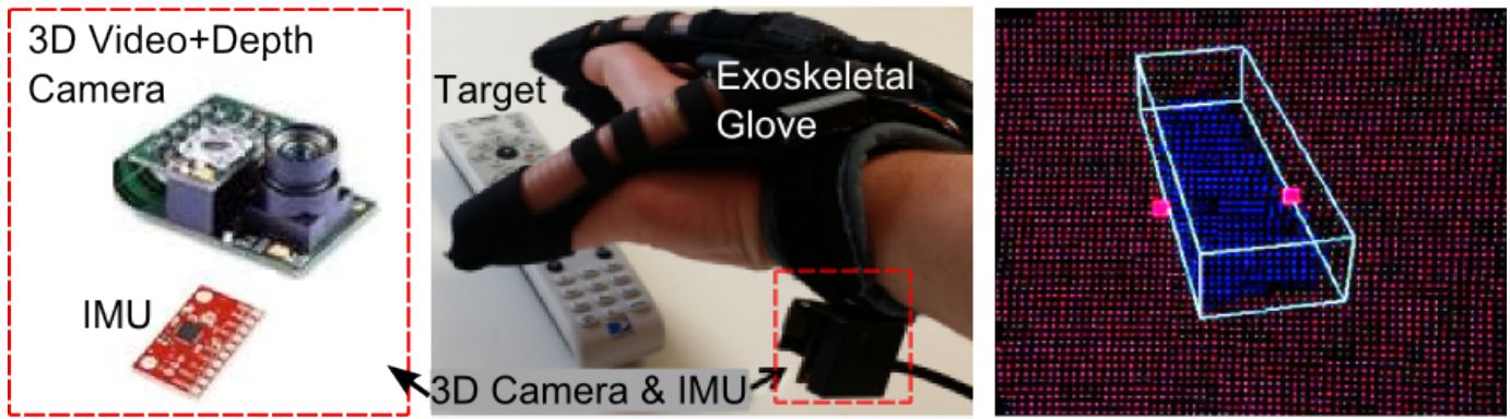
Fig. 1. Real-time 3D object sensing. (Left) 3D depth+video camera and IMU; (Middle) Exoskeletal glove mounted with a depth camera and IMU looking at the target object; (Right) Processed depth image: red pixels = table top, blue = object; white = bounding box of object from segmented object and PCA; pink dots = target grasp points determined as opposition points on minor axis parallel to table.
