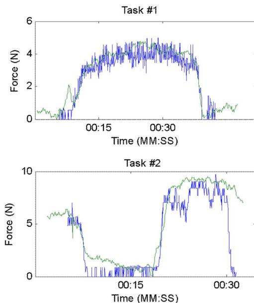
Fig. 5: Agreement between sensorized cannula (blue) and ATI (green) measurements during static retraction tasks
