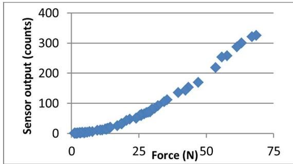
Fig. 4: Calibration curve for one sensor on a strip
