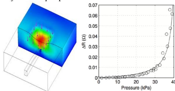
Figure 1: Soft Sensor response to pressure [1]
