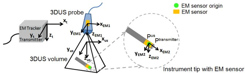
Fig. 2. Coordinate transformations for instrument tip location
