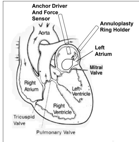
Figure 2: The prototype beating heart mitral valve annuloplasty uses two instruments inserted through the left atrial appendage. One instrument deploys anchors that secure a stiff ring to the annulus to reshape it. Note that the anchor driver approaches along the valves axis, which corresponds to the valves major component of motion.
