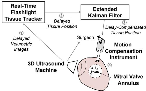
Figure 1: The motion compensation system uses 3D ultrasound imaging to automatically synchronize the motion of an actuated, handheld surgical instrument with a tissue target. Circled numbers indicate the order of data flow through the system (1–3) and the resultant tracking position of the motion compensation instrument (4).
