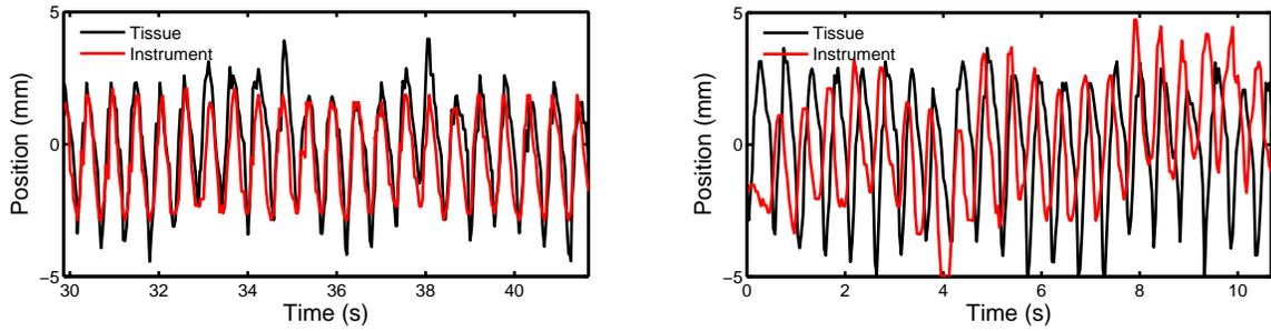
Figure 10: *In vivo* tracking examples conducted with the motion compensation system (A) and manually (B). The manual tracking example is the last and best attempt, after the surgeon had two training trials. The relative positional offsets between the instrument and tissue target are removed for clarity.
