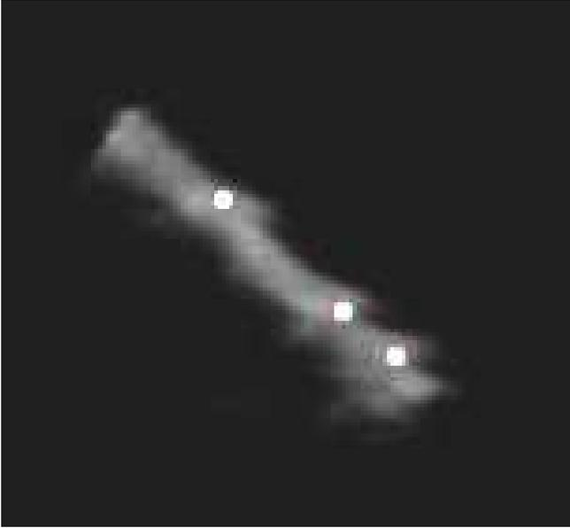
Fig. 4. 3D ultrasound image of a surgical instrument in a water tank. The results of the passive marker tracking is indicated by the white dots.
