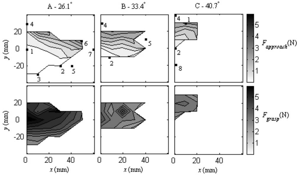
Fig. 9. Forces on the PVC cylinder object during the approach (top row) and grasp (bottom row) phases for the three object locations (columns). Labeled configurations correspond to the behavior indicated in Table I.
