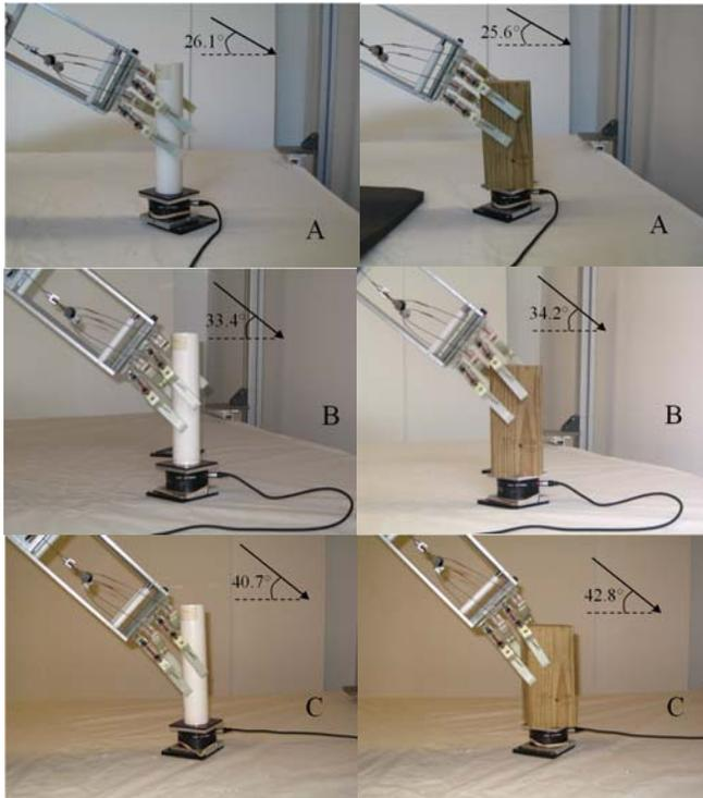
Fig. 8. Two target objects (PVC cylinder of radius 24mm and wood block with square cross-section 90mm side length) at three locations (A, B, and C). Note the differences in approach angle for the locations, the main factor affecting the force and grasp space results.
