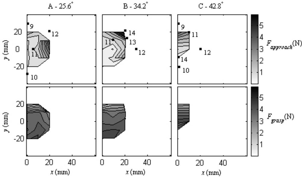
Fig. 10. Forces on the wooden block during the approach (top row) and grasp (bottom row) phases for the three object locations (columns). Labeled configurations correspond to the behavior indicated in Table II.
