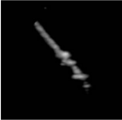
Fig. 6 - 3D ultrasound image of instrument showing marker ridges.
