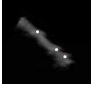
Fig. 6. 3D ultrasound image of a surgical instrument in a water tank with white dots indicating tracked passive markers.
