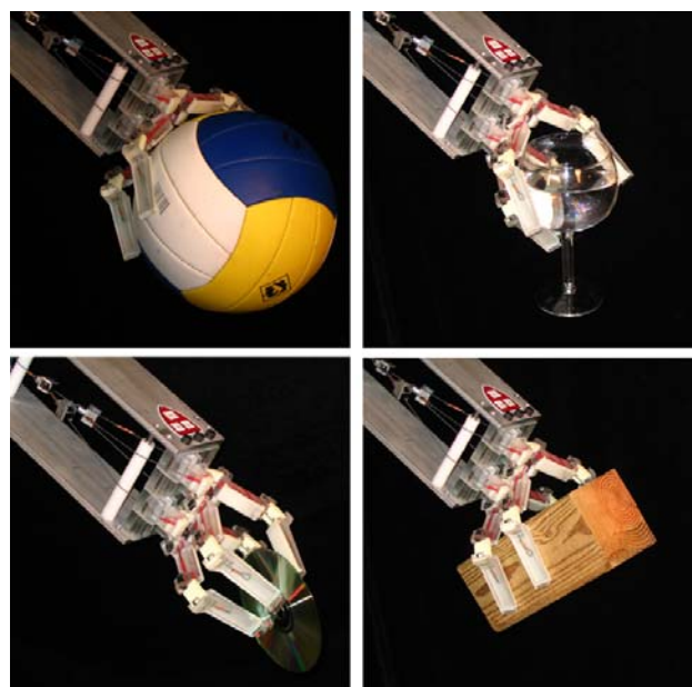
Fig. 2. Four-fingered SDM grasping a volleyball, a wine glass filled with water, a compact disc, and a large wood block.
