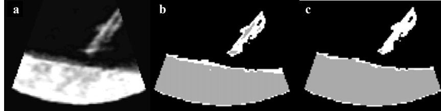
Figure 1: Tank data: (a) a slice of a 3D US image of an acetabular rod approaching a tissue sample in a water tank; (b) detection results without spatial information, where the instrument is shown in white and the tissue in grey; (c) detection results employing spatial information.
