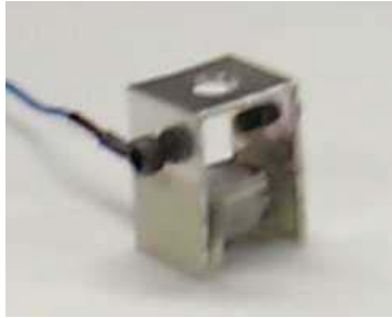
Figure 3: Close-up of the manipulandum object fitted with force sensor
