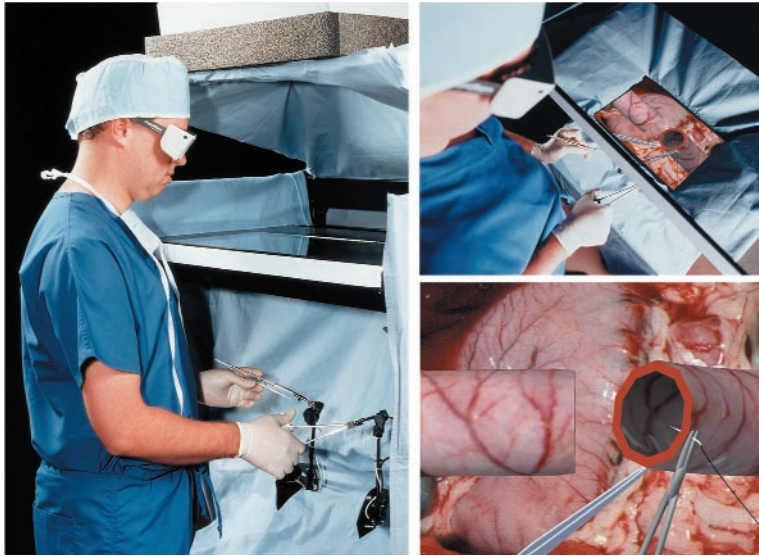
Figure 11 Surgical simulation training system for end-to-end anastomosis procedures. ( Left image ) Using a needle holder and forceps attached to force-feedback devices, the user can grasp, poke, pluck, and suture flexible vessels. ( Upper right ) A mirror arrangement superimposes the 3-D image of the operative field in the correct position relative to the surgeon's hands. ( Lower right ) Mechanics-based models generate forces and images that change realistically in response to contact. (From R O'Toole, R Playter, T Krummel, W Blank, N Cornelius, et al. Assessing Skill and Learning in Surgeons and Medical Students Using a Force Feedback Surgical Simulator . In Proc. Med. Image Computing and Comp.-Assisted Intervention , Cambridge, MA, 1998, p. 404. Ed. WM Wells, A Colchester, S Delp. Berlin: Springer-Verlag. Reprinted with permission.)
